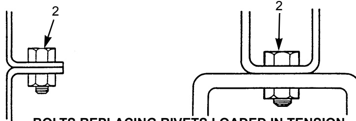
BOLTS REPLACING RIVETS LOADED IN TENSION
